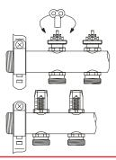
Adjust the flow volume by turning the spindle. The actual flow volume can be viewed on the supply-sided flowmeter.
