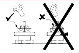
The fine thread of the adjusting spindle must not be seen above the edge of the size 19 hex! Based on closed status, the valve is open (full flow) after 2 1/2 - 3 turns to the left.
