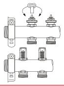
Adjust the required flow volume by turning the regulation spindle to the left.
